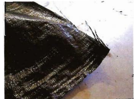
Here is an example of inexpensive fabric that will not do too much as a weed barrier and will tear quite easily.
